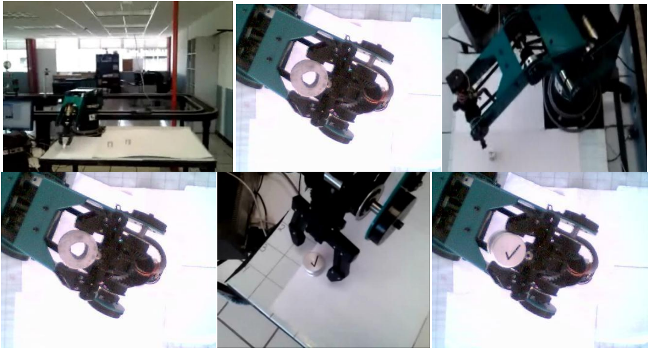
Fig 10: Sequence of Scorbot-Er 4u in your trajectory calculated through of MED, also the selection and classification of objects.
