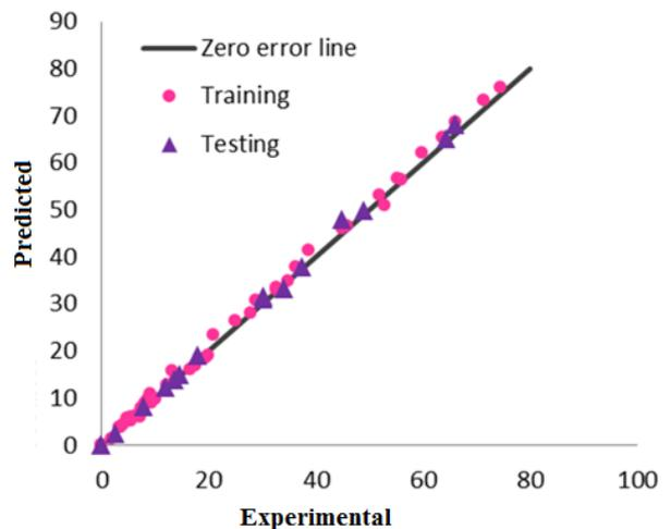
**Fig. 4: The values of glucose concentration predicted versus experimental values for training and testing dataset using ANN**
