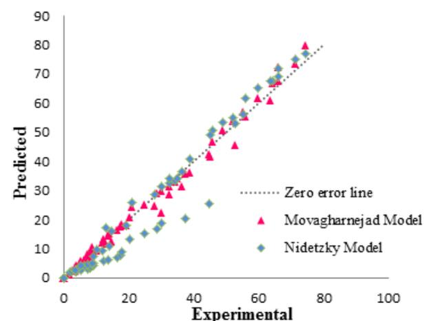
Fig. 2: The values of glucose concentration predicted by two mathematical models versus experimental values
