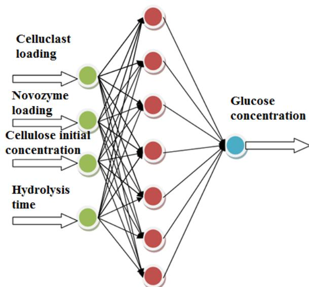
Fig. 1: Architecture of ANN used in developing model
