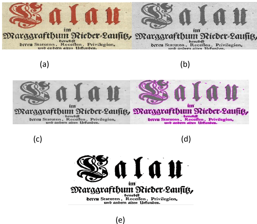
Figure 4. a) Original image taken from DIBCO 2009 dataset b) image obtained after edge enhanced diffusion operation c) image obtained after applying split bregman algorithm d) contour formed using level set method e) segmented and binarized output
