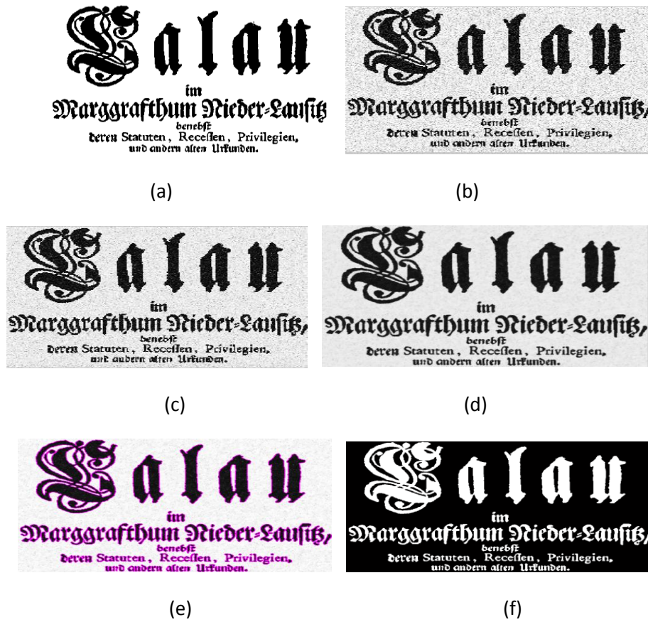
Figure 4. a) Original image taken from DIBCO 2009 dataset b) Gaussian noise added to the image c) image obtained after edge enhanced diffusion operation d) denoised image obtained after applying Split Bregman algorithm e) contour formed using level set method f) segmented and binarized output.
