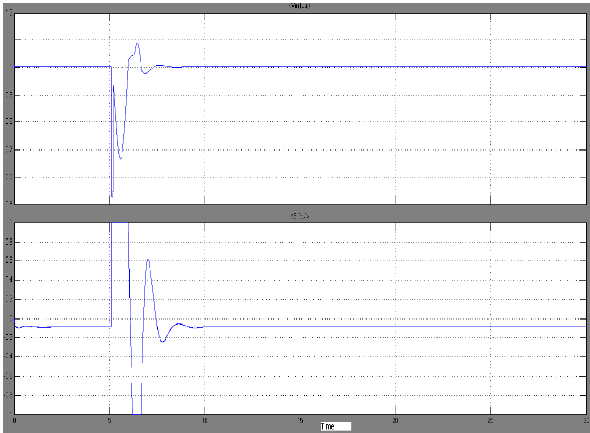
Fig 10: Signals Observed on ‘SVC’ Scope With SVC
