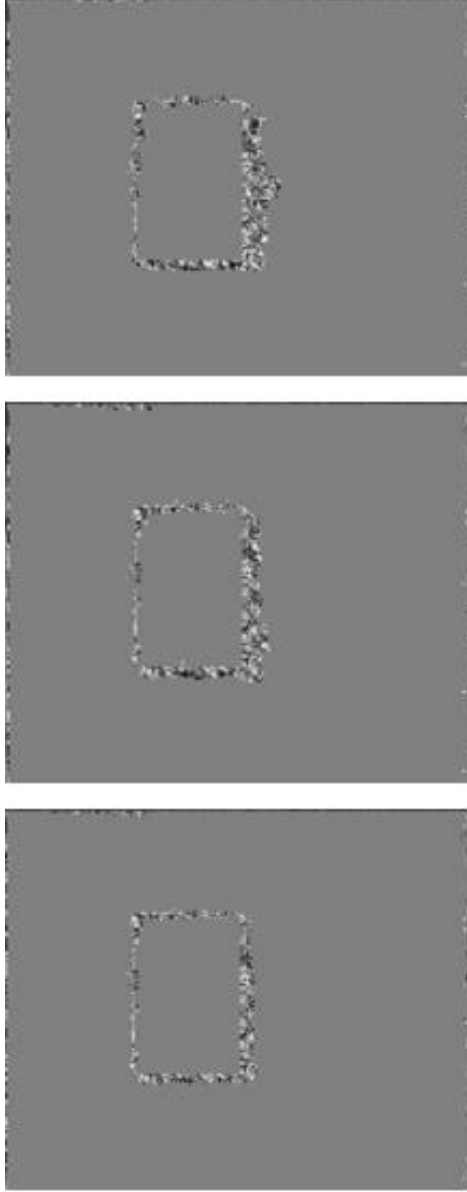
Fig 3: Motion error obtained for the Wiener filter (top), A_{RLS}=\lambda I (middle) and A=\text{diag} \{\lambda_1, \dots, \lambda_N\} (bottom) for the "Synthetic" sequence with SNR=20\text{dB} .
