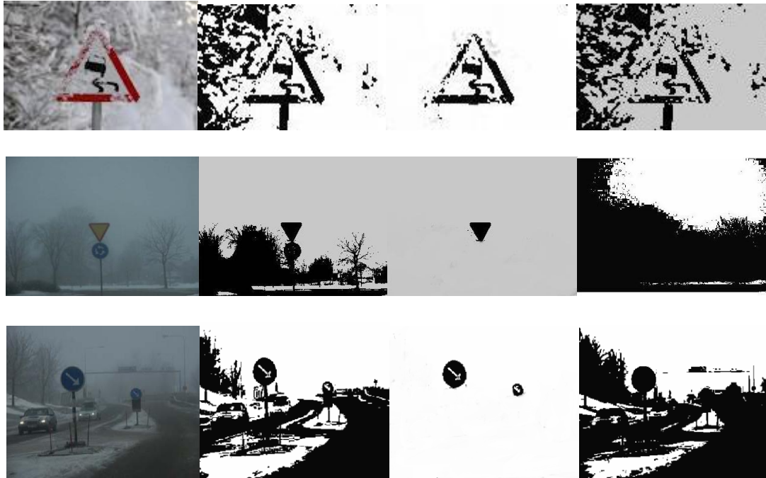
Fig 3: Segmentation result. First column: Original images. Second column: Segmented images using MFCM algorithm. Third column: Candidate ROIs. Fourth column: Segmented images using FCM algorithm.
