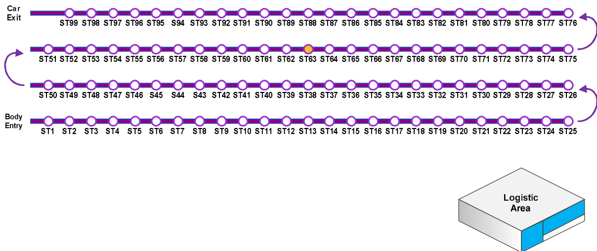
Fig 1: Station sequencing and layout in production area
