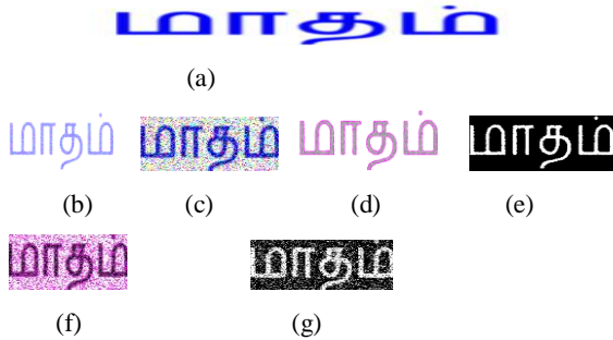
Fig 7: Results of Bresson's level set method for binarization of noisy data (a) Original data (b) Original data in (a) embedded with Gaussian noise of 60% intensity (c) Original data in (a) embedded with impulse noise of 20% intensity (d) Contour drawn by Bresson's method for 'Gaussian' noise image (e) Result for binarization by Bresson's method for 'Gaussian' noise image (f) Contour drawn by Bresson's method for 'impulse' noise (g) Result for binarization by Bresson's method for 'impulse' noise.
