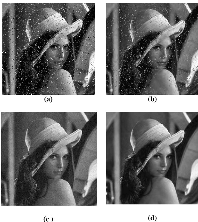
Fig. 5: Denoised images using BBEMD approach with 2 IMFs filtered: a) Noisy image with impulsive noise 10%, b) Denoised image with BBEMD(2IMFs), c) Noisy image with Gaussian noise \sigma=10 , d) Denoised image with BBEMD(2IMFs) .
