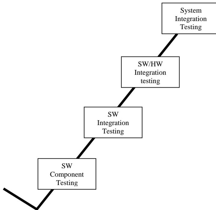
**Figure 3 : Right Branch of the V Model for embedded system**
