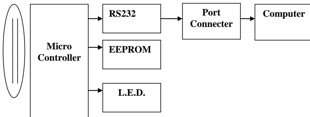
**Figure 2 : Block diagram of ECG system**
