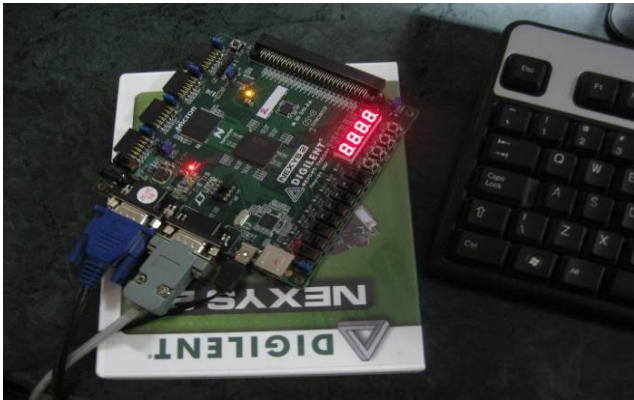
Figure 16: Digilent Nexys2 FPGA Board with VGA cable connected Through Serial (RS-232) Communication
