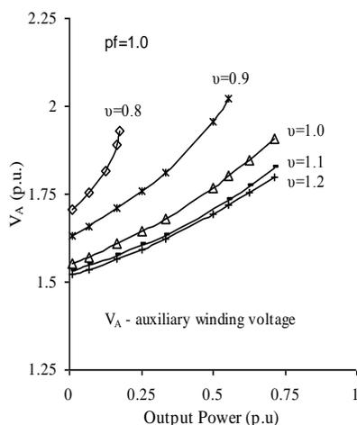
Fig. 7. Variation of  $V_A$  with output power to keep  $V_t$  constant at 1p.u.
