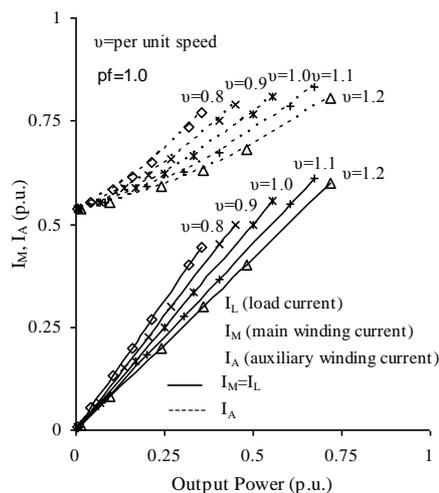
Fig. 9. Variation of  $I_M$  and  $I_A$  with output power to keep  $V_t/v$  constant at 1p.u.
