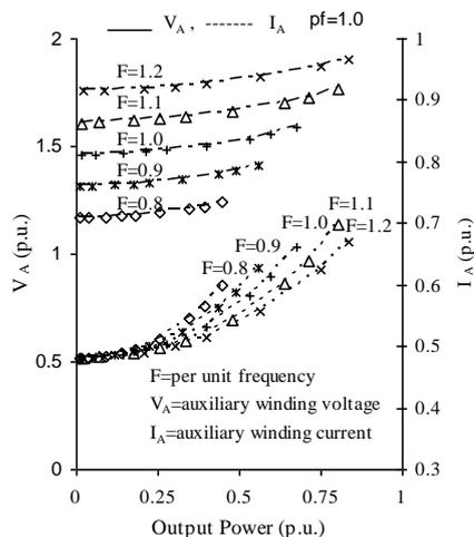
**Fig. 12. Variation of  $V_A$  and  $I_A$  with output power to keep constant air gap flux ( $V_g/F=1.0$ ) for different values of  $F$ .**
