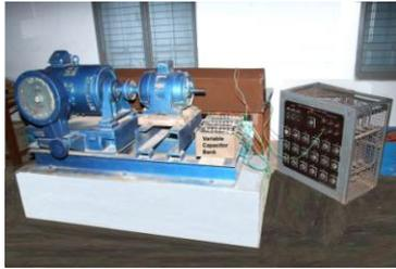
Fig.4. Photograph of the single-phase two winding SEIG.
