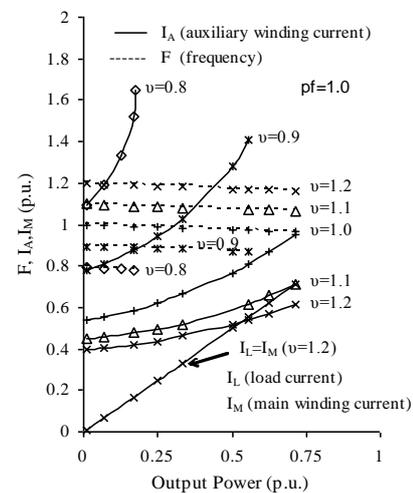
Fig. 6. Variation of  $F, I_A$  and  $I_M$  with output power to keep  $V_t$  constant at 1p.u.
