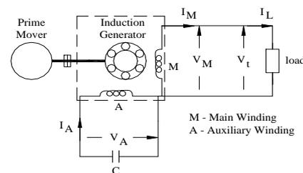
Fig. 1 Schematic diagram of capacitor excitation of two winding single phase self excited induction generator
