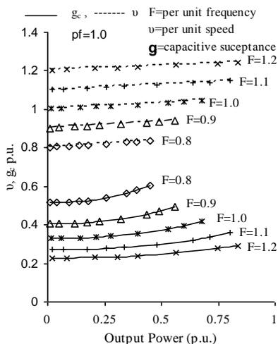
**Fig. 11. Variation of  $v$  and  $g_c$  with output power to keep air gap flux constant i.e.,  $V_g/F$  constant at 1p.u. (for different constant value of  $F$ ).**
