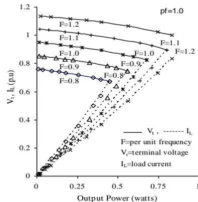
**Fig. 13. Variation of  $V_t$  and  $I_L$  with output power to keep constant air gap flux ( $V_g/F=1.0$ ) for different values of  $F$ .**
