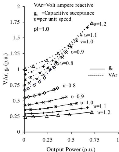
Fig. 8. VAR and  $g_c$  required at different output power to keep  $V_t/v$  constant at 1p.u.
