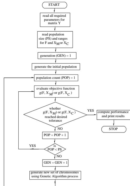
Fig. 3. Flow chart for minimization of the objective function using genetic algorithm (GA).
