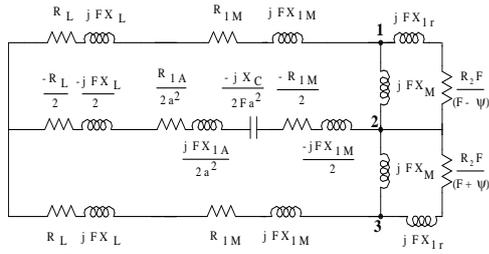
Fig. 2. Equivalent circuit of single-phase two winding self-excited induction generator.
