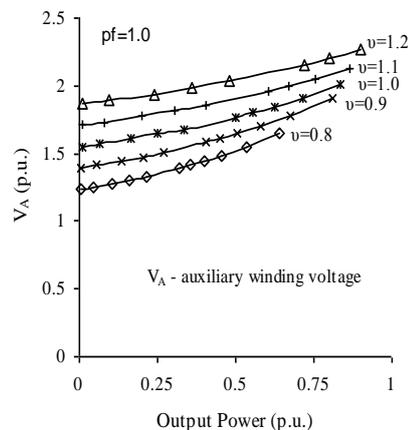
Fig. 10. Variation of  $V_A$  with output power to keep  $V_t/v$  constant at 1p.u.
