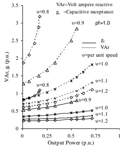
Fig. 5. VAR and  $g_c$  required at different output power to keep terminal voltage  $V_t$  constant at 1p.u.
