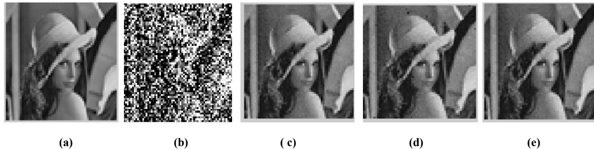
Fig 12: (a) Original lena (b) Lena image corrupted by Gaussian noise mean zero and variance 0.2 (c) Restored image using canny (d) Restored image using sobel (e) Restored image using prewitt
