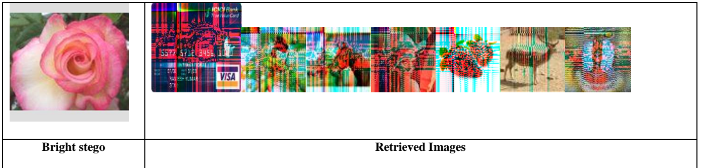
Figure 8: Effect of brightness attack on stego generated using DCT
