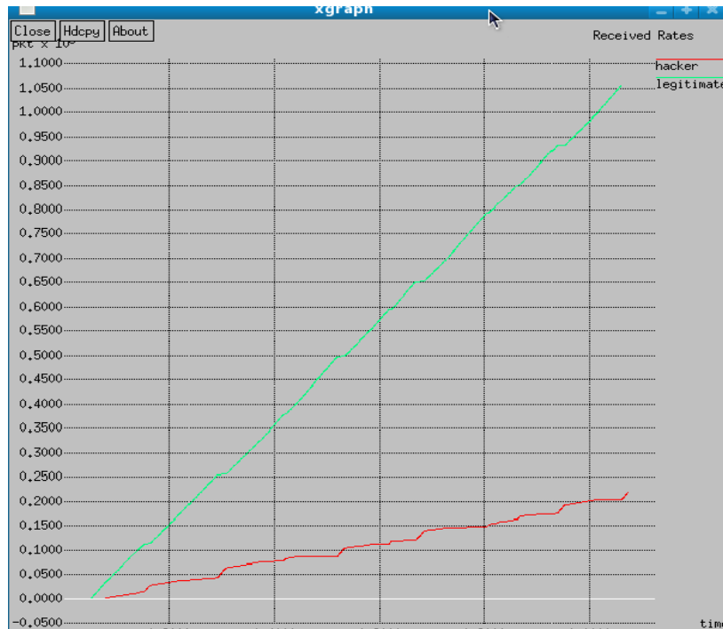
Fig. 2. Time vs received packets of legitimate and attack packets.
