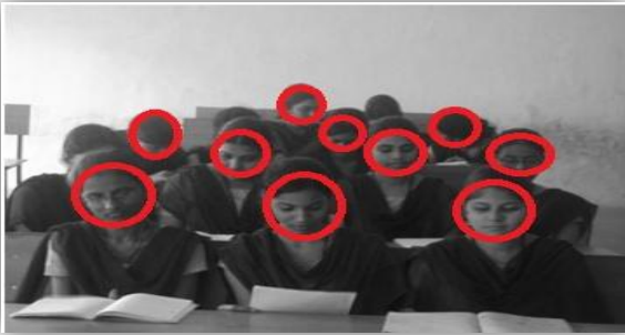
Fig 5: Output of the face detection algorithm this could not detect all faces
