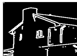
Segmentation using sobel e_{rms}=212.1175 (Best results)
