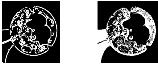
Segmentation using sobel e_{rms}=276.2977 Segmentation using thresholding e_{rms}=276.1223 (Best results)
