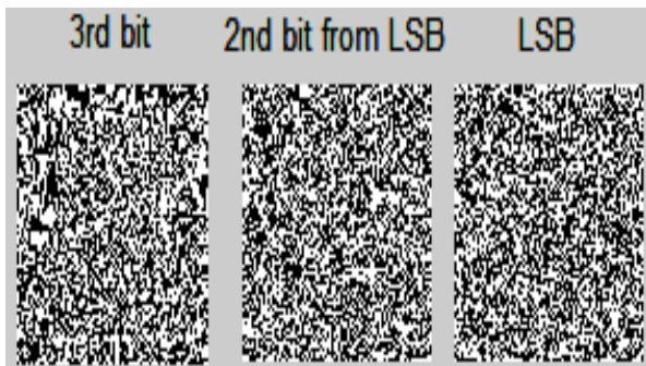
Figure 5. Three LSB Bit planes of the Original Lena Image
