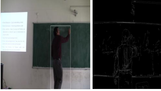
Figure-3: (a) Tracking of an object (b) Image after edge detection.
