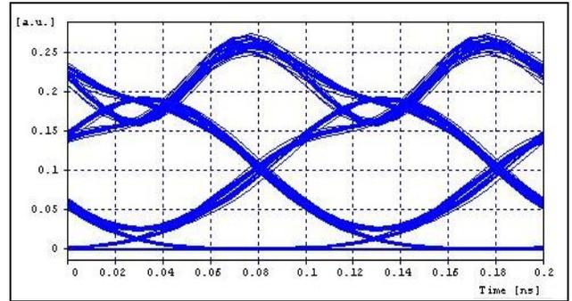
**Fig. 4 (a) Eye Diagram for 60 Km, NRZ Coding**
