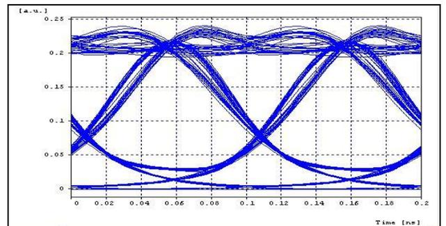
**Fig. 4(b) Eye Diagram for 60 Km, RZ Coding**
