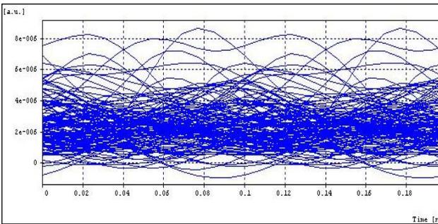
**Fig. 3(b) Eye Diagram for 10 Km, MMF**
