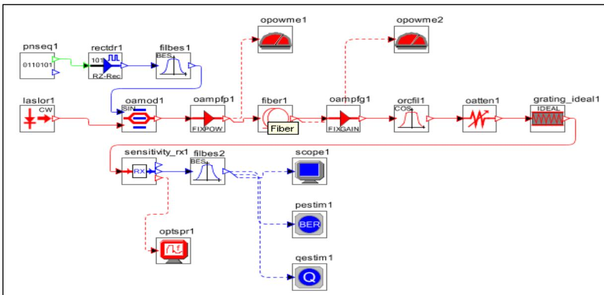
**Fig. 2 Block Diagram of SMF Optical Fiber Link with NRZ Scheme**
