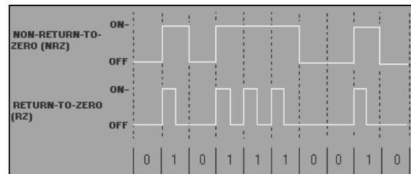
Fig. 1 RZ vs. NRZ Coding Scheme
