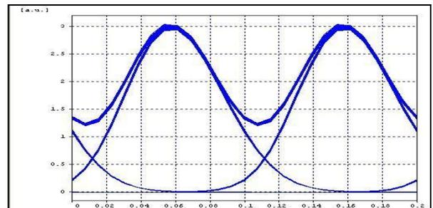
**Fig. 4(c) Eye Diagram for 10 Km, RZ Coding**
