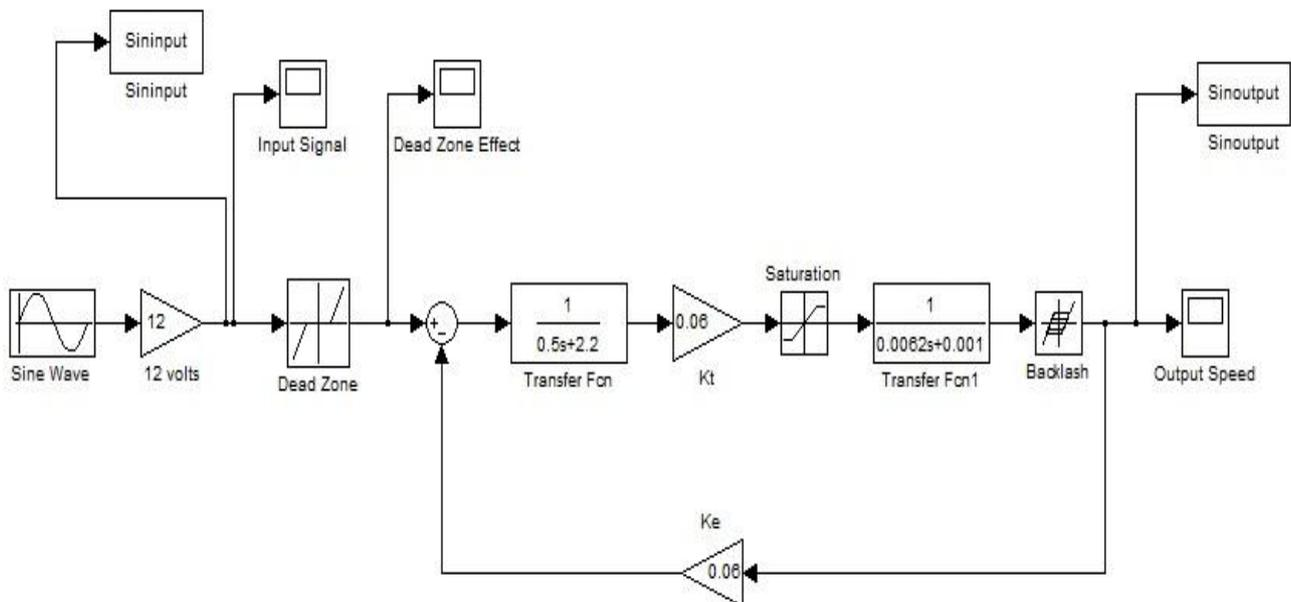
**Fig 4: DC Servo Motor Model (Simulink Environment)**
