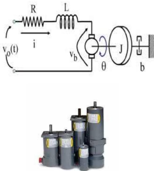
**Fig 2: Servo Motor Circuit Diagram and original DC Servo Motors (Courtesy of Baldor Servo Motors)**
