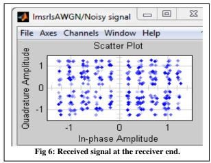
Then the received signal compared with the desired signal and equalized it with respect to the desired signal. This process is done by adaptive equalizer which may be LMS or RLS equalizer. The received signal equalized by LMS equalizer then the scatter plot of the output signal looks like as Fig 7.
