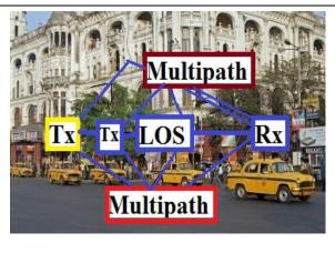
Fig 2: Rician Fading Channel with existing one LOS
