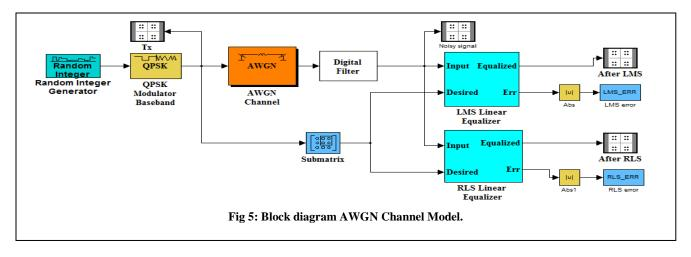
The AWGN channel model is referred in v2v communication where no multipath or echo can affect the transmitted signal. In this channel only some noise is added with the transmitted signal, which is received by the receiver side vehicle.
