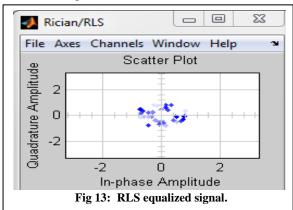
In this case for the Rician fading model, it is again prove that RLS equalizer is more efficient to reduce the error.
