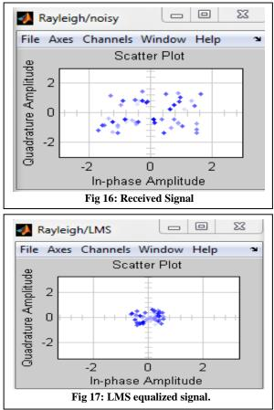
Similarly as the case I & case II RLS equalizer takes less time to equalize the noisy signal. Fig 17 is the scatter plot of LMS equalized signal. RLS equalized signal of Rayleigh fading channel model is shown in the Fig 18.
