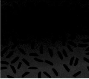
**Fig 9: Approximated non-uniform background image extraction using histogram equalization**
