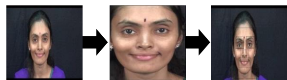
Fig 3: (a) Detection of Face from 2D Frame; (b) Detected faces components.
