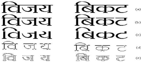
Figure 5: Preprocessed Images (a) Original, (b) segmented (c) Shirorekha removed (d) Thinned (e) image edging
