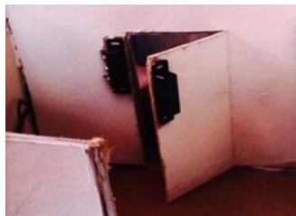
Fig. 6 Entry detection using Reed Switch
