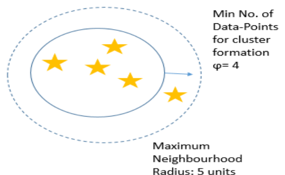
Figure 4. Visualization of Density based clustering with sample constraints for Min. points and maximum cluster radius being (4, 5 units) respectively.
