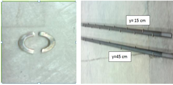
Fig. (4): Semi circular disk baffles with spacing between baffle and another (y=15 and y=30) cm.
