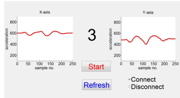
Figure 8: The predicted digit is displayed on the GUI. It also plots the filtered X and Y axis accelerometer readings.
