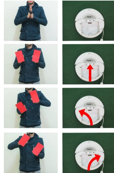
Fig 2: The predefined signs from the user for controlling the robot.
