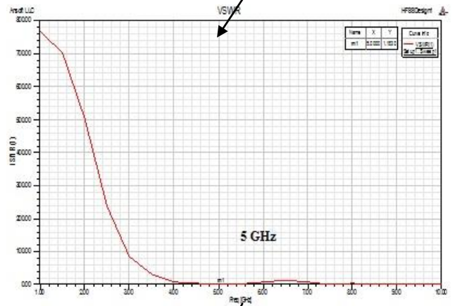
Fig 6: VSWR of Rectangular patch antenna with rectangular ground
