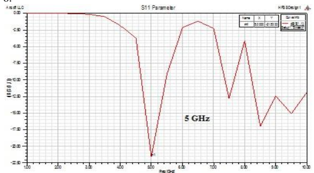
Fig 5: S11 parameter of Rectangular patch antenna with rectangular ground
