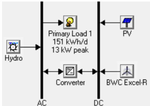
Fig 5. Proposed Solar-Wind-Hydro Hybrid Electrical Supply
