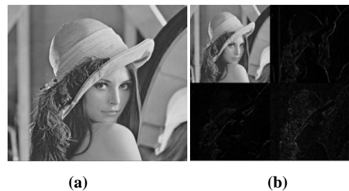
Figure 4: (a) Lena image, (b) Image after the first-order 2-D Haar-DWT [14]
