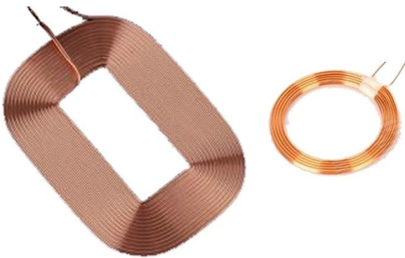
Fig 3. Different sizes and shapes of inductor coil
