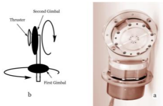
Fig 1: a. biaxial gimbal scheme [7], b. gimbal platform sample
