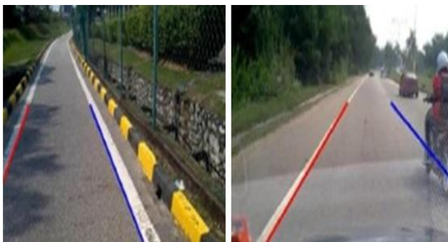
Figure 9: a) Detection in shadows b) Detection in vehicles [19]
