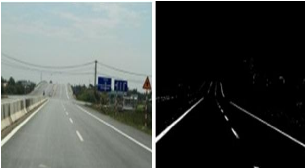
Figure 8: a) Input Image b) Detected Lanes [2]
