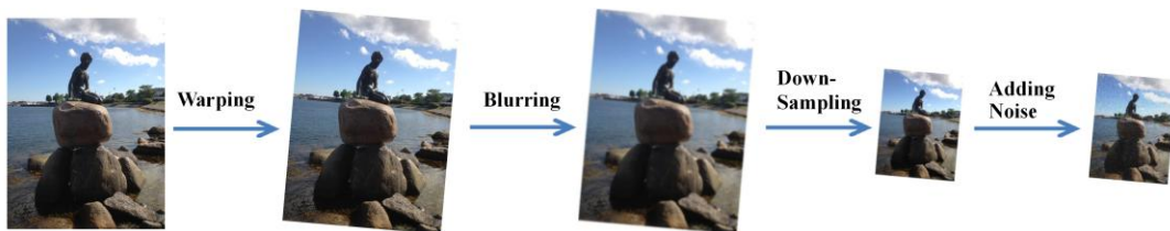
Fig. 1 The imaging model used in most superresolution algorithms[51]
