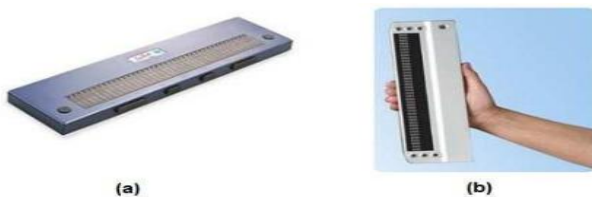
Fig. 2: (a) Braille line Keika. (b) Braille Line SuperVario40.
