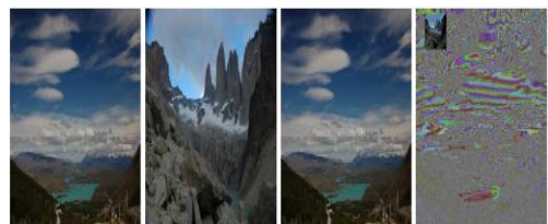
Fig.1.1 a) Cover image b) Secret image c) Stego image d) Lower bits of Stegified Image
