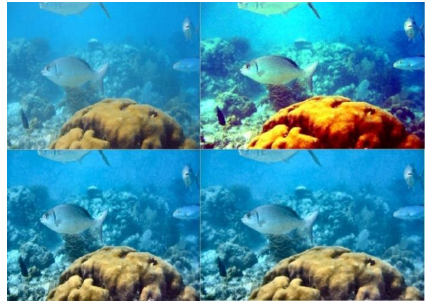
Figure 1: Comparison of methods on. Upper left: original underwater image. Upper Right: Mix CLAHE image. Bottom left: L*A*B CLAHE image. Bottom Right: New Enhancement image
