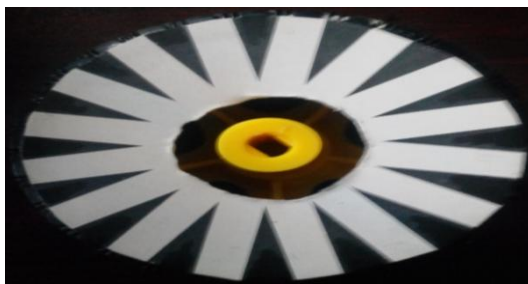
Fig5. Encoder disk mounted on a wheel
