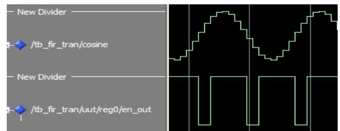
Fig. 10 Simulation results for register with subword based clock gating
