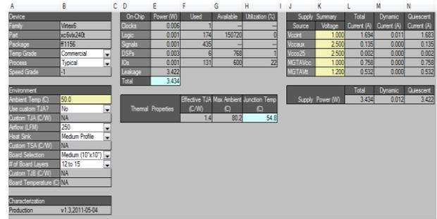
Fig. 13 Xpower report for FIR architecture with proposed clock gating
