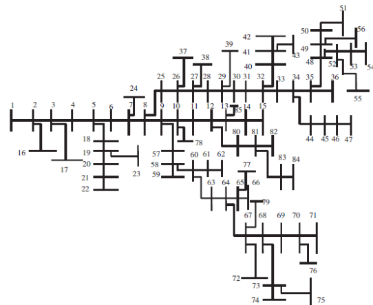
Fig 5 Single line diagram for 85-bus radial distribution system
