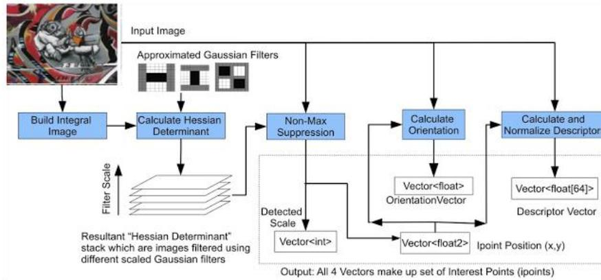
Fig.1.2. the work of SURF
