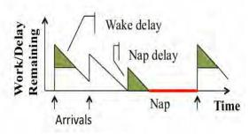
Wake delay: This is the time duration taken by the processing unit to turn on all it's services from the state of nap. Till the wake delay ends, the work remains fixed.
