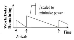
Explanation: Initially, a certain amount of work is taken in the cluster and when it ends, it creates an idle time state for the servers, we have DVFS to scale the voltage and frequency such that the time taken by the servers can be modified and such intermediate idle states are avoided. This is possible only when the upcoming work's arrival time is predicted or known. So, for each work arrival the previous work is stretched till the new work is arrived.
