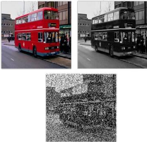
Fig 1: The process of adding salt and pepper noise to the color image
