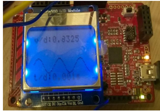
Fig 5: Sine wave of 1.5 Vp-p and frequency of 1 KHz
