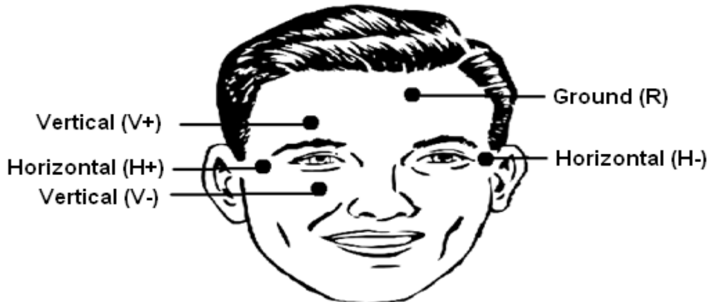
Fig 1: Electrode Placement for EOG signal acquisition.
