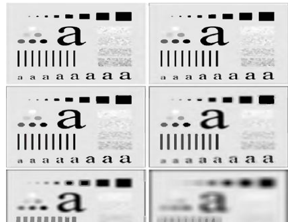
Fig 1: Smoothing of Image by Low Pass Filters
