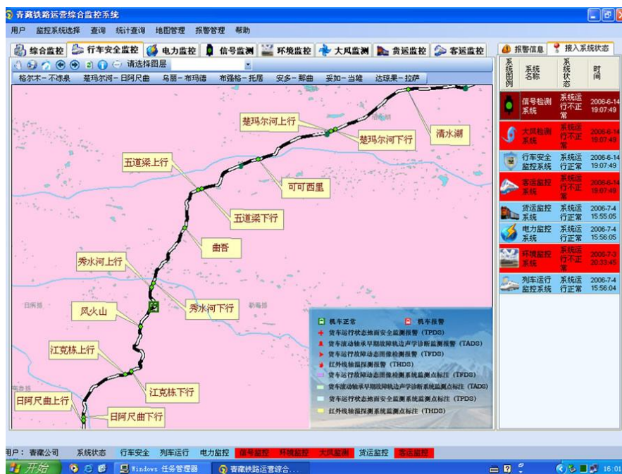
Fig 4: GIS based Qinghai-Tibet Railway Bureau comprehensive monitoring system (Source: Enterprise GIS Helps Safeguard the Qinghai-Tibet Railway)
